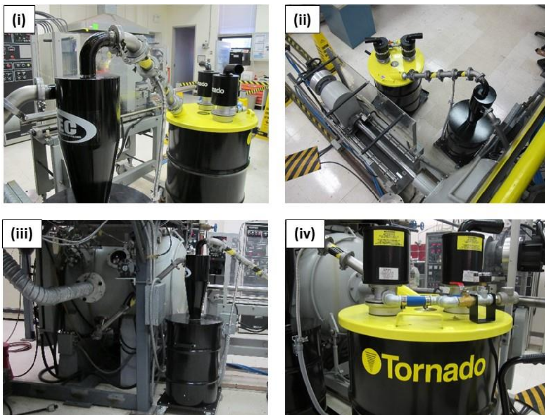
Figure 24. Ruwac cyclone and Tornado pneumatic vacuum system connected in series for dry collection at room temperature: (i) side view of setup; (ii) overhead view of setup; (iii) exhaust exits chamber and enters cyclone; and (iv) exhaust exits cyclone and enters twin pneumatic suction pumps.
